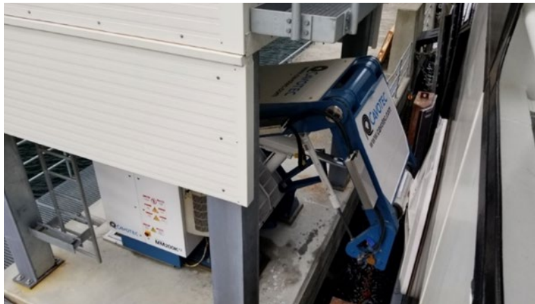
Figure 7: Cavotec MoorMaster Automated Vacuum Mooring System
