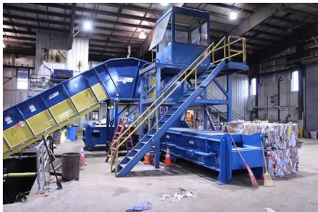
Figure 5: Side view of baler as well as bales from this machine.
