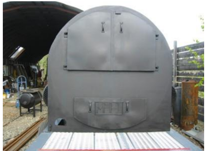
Figure 7: Skid-mounted burn unit.
