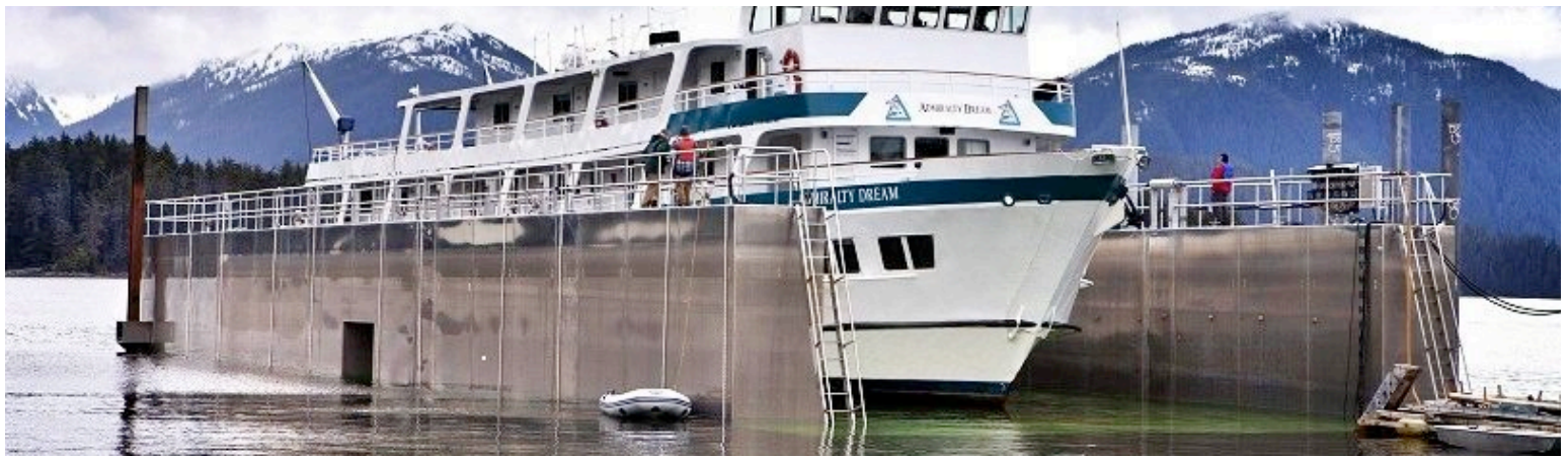
Allen Marine Inc.'s Admiralty Dream in a floating dry dock made of marine grade aluminum. Both the dry dock and ship were built by Allen Marine in Sitka.
